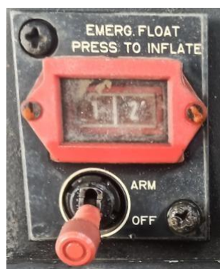
Fig 4: Float Switch in OFF position
